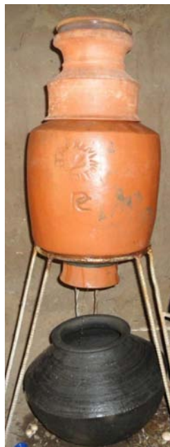
Figure 1: Final product of INREM's filter on location in Jhabua
